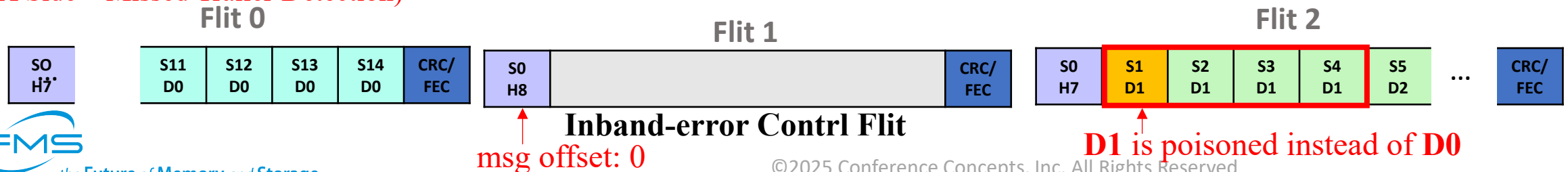
• Figure 4: Received 3 256B-Flits (RX Side – Missed Trailer Detection)
