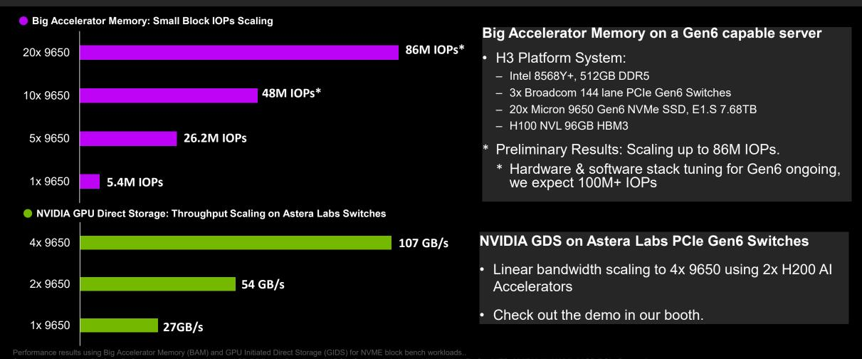
System under test: H3 Platform PoC system, 1x Intel 8568Y+, 512GB DDR5, 3x Broadcom A0 PCIe Gen6 switches, 20x Micron 9650 E1.S 7.68TB, NVIDIA H100NVL-96GB PCIe Gen5x16 BaM performance testing completed by Micron's Data Center Workload Engineering team in the Longmont, CO lab. GDS testing completed by the Astera Labs performance engineering team in San Jose, CA.
