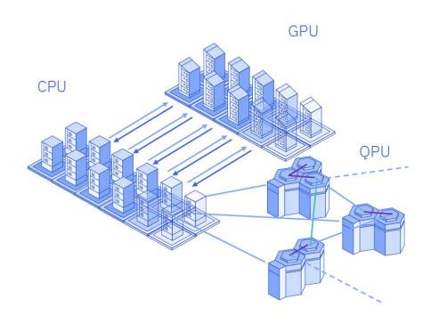
Quantum-centric supercomputing utilizes a modular architecture to enable scaling.
