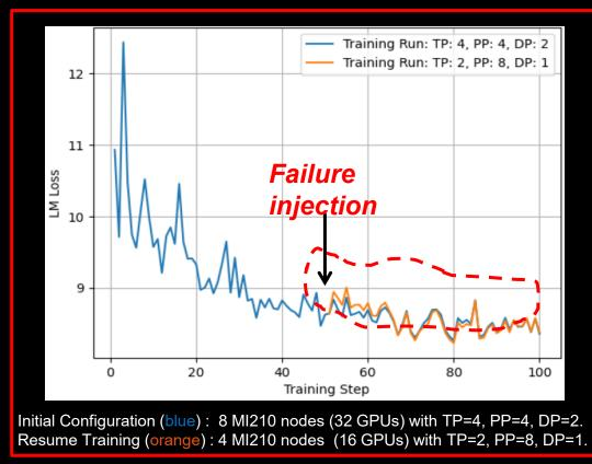
UCP enables failure recovery with resource rebalancing (GPU shape, parallelism) without compromising training accuracy.
