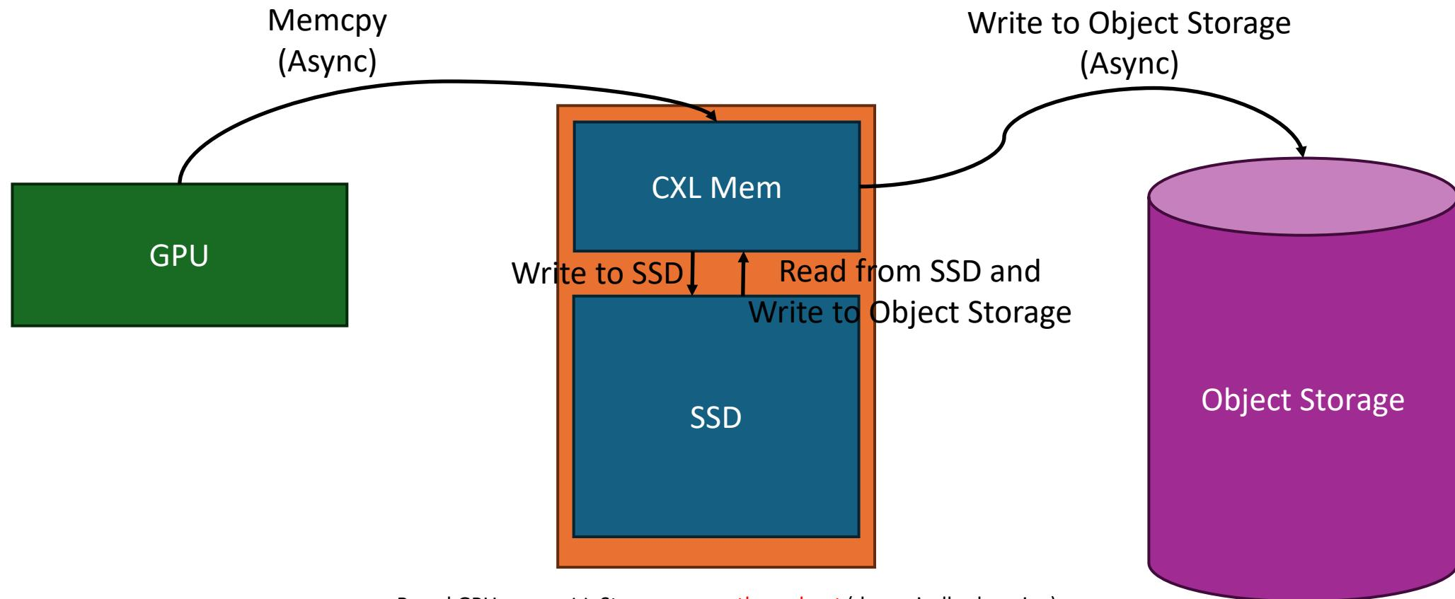
Based GPU server ↔ Storage server **throughput** (dynamically changing), policy determines whether to write/keep checkpoint data in local SSD or move to remote object storage.
