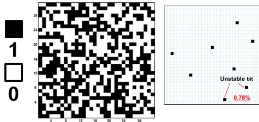
After reading 10,000 times, only two unstable bits were observed.
