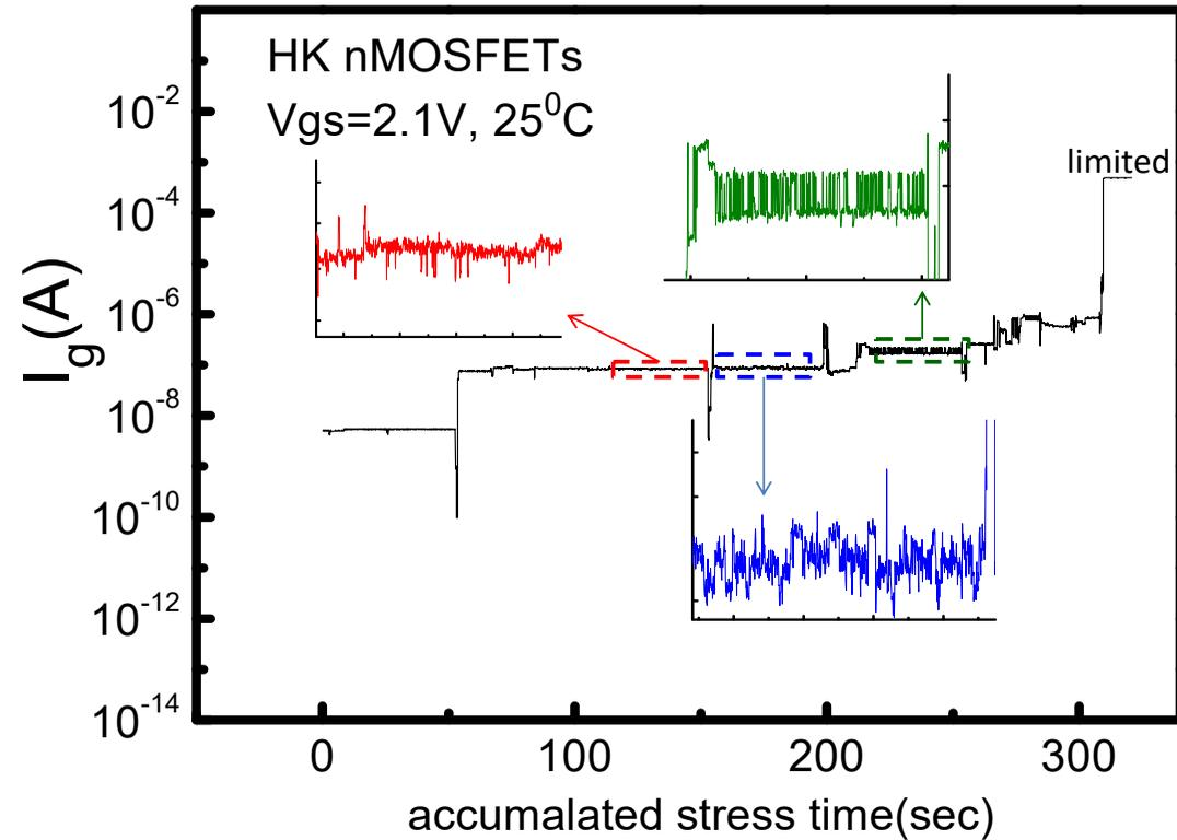
Measuring trap generation as a function of time, we may trace the leakage path.
