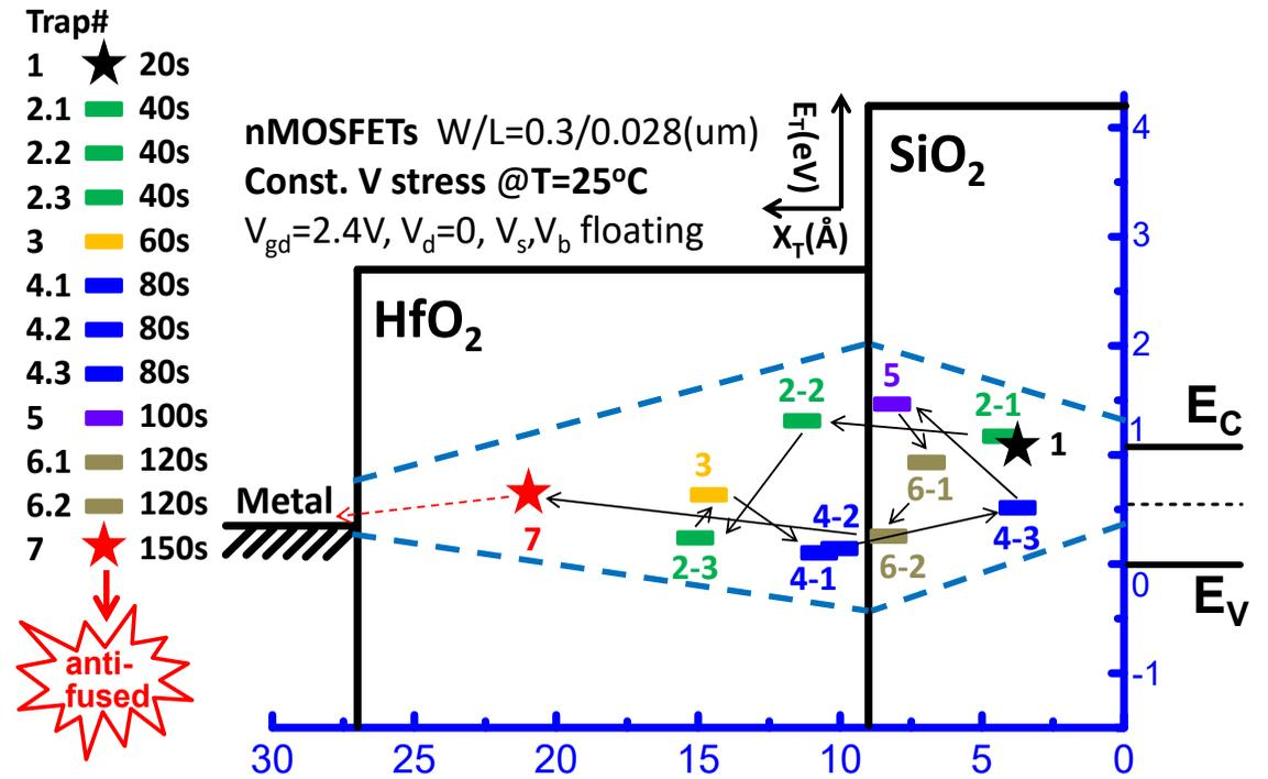
**Hard-breakdown: the breakdown path behaves as a snake path.**
