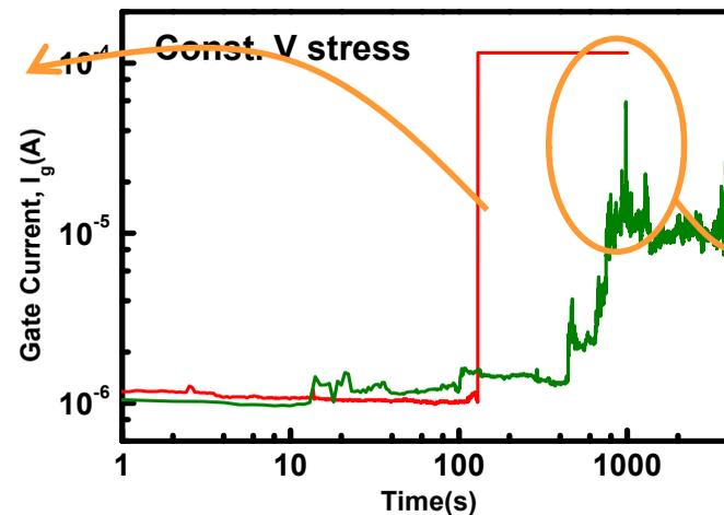
**Soft-breakdown: the breakdown path forms as a spindle shape.**
