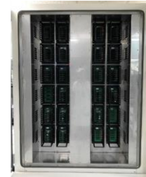
ATP Proprietary Coach-Gym Testing System for I-Temp testing (-40°C to 85°C)
