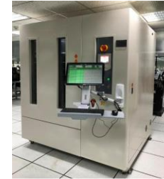
ATP Proprietary Coach-Gym Testing System for I-Temp testing (-40°C to 85°C)
