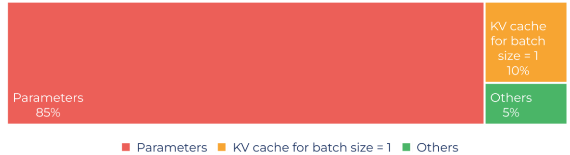
Storage allocation for Llama2 7GB (FP16) in inference, by number of users on a single Nvidia H100 80GB
