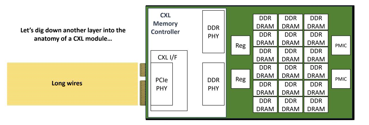
CXL modules assume a very long PCIe bus requiring high current drivers
