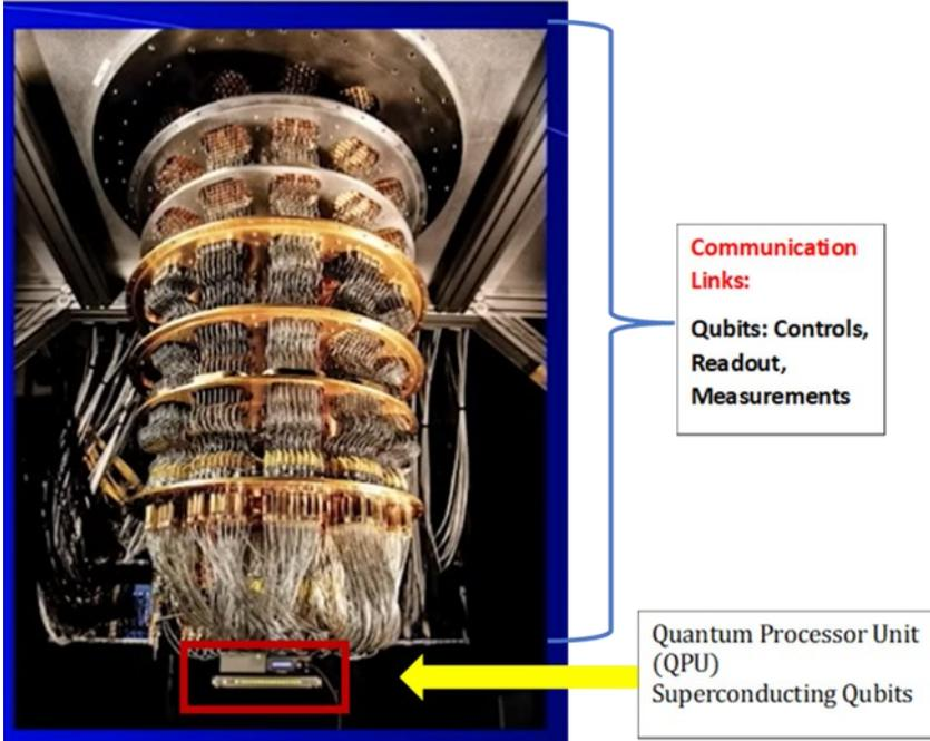
Fig 4: Typical Quantum Computer Communication Links,
