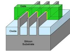
Tri-Gate transistors can have multiple fins connected together to increase total drive strength for higher performance
