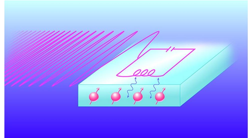
Superconducting circuit resonator and a silicon chip embedded with bismuth atoms. Chirped microwave pulses transfer quantum information back and forth between the resonator and the bismuth atoms, stored in the atoms spin states
