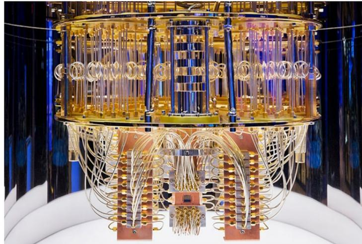
The innards of an IBM quantum computer show the tangle of cables used to control and read out its qubits. Credit: IBM
