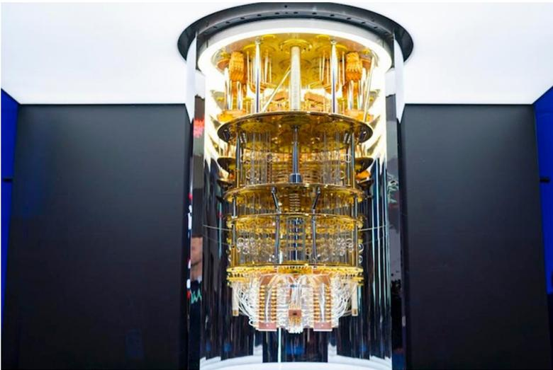
QPU and Cables within Dilution refrigerator, IBM Quantum Computer
