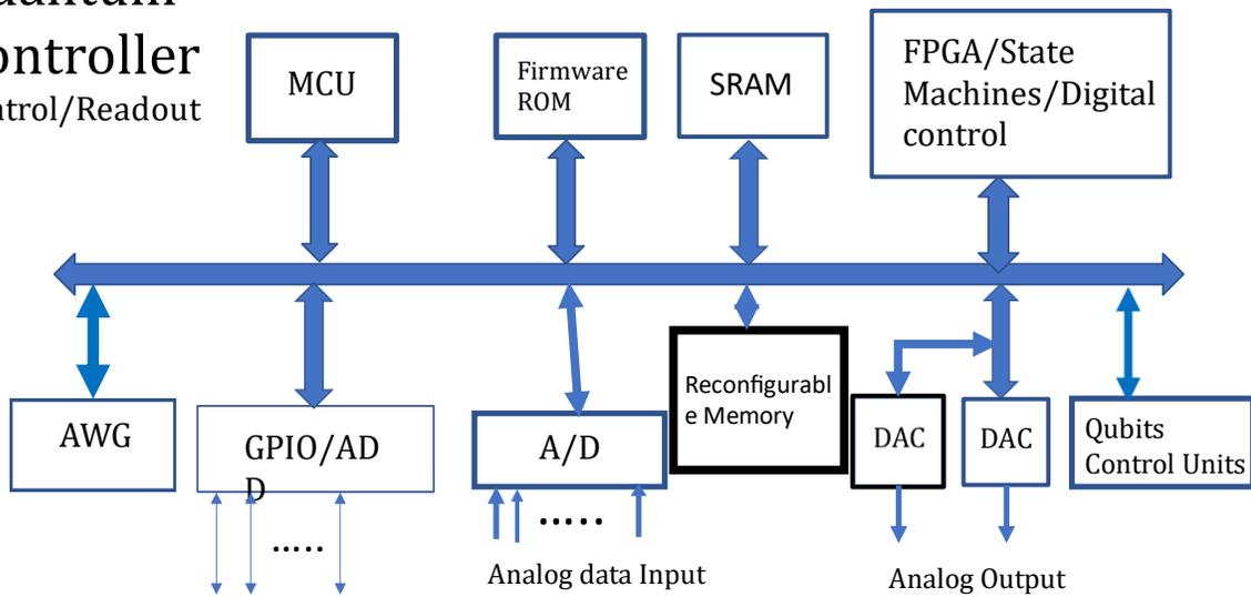
Fig 3. Quantum controller – Control/Readout
