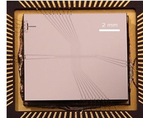
Surface-Electrode Trap Chip
