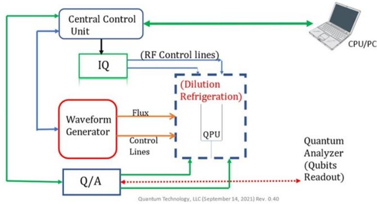
Fig 2: Quantum Computer Controller Block diagram
