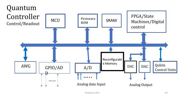
Fig 3. Quantum controller - Control/Readout
