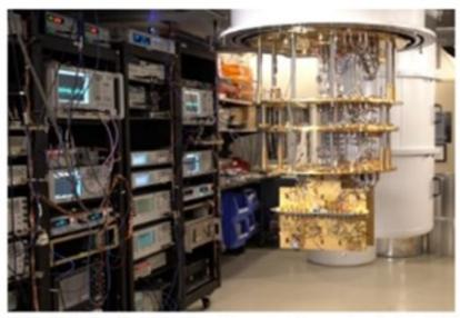
Source: MIT/Lincoln Laboratory Quantum Computer (Super-Conducting Qubits)
