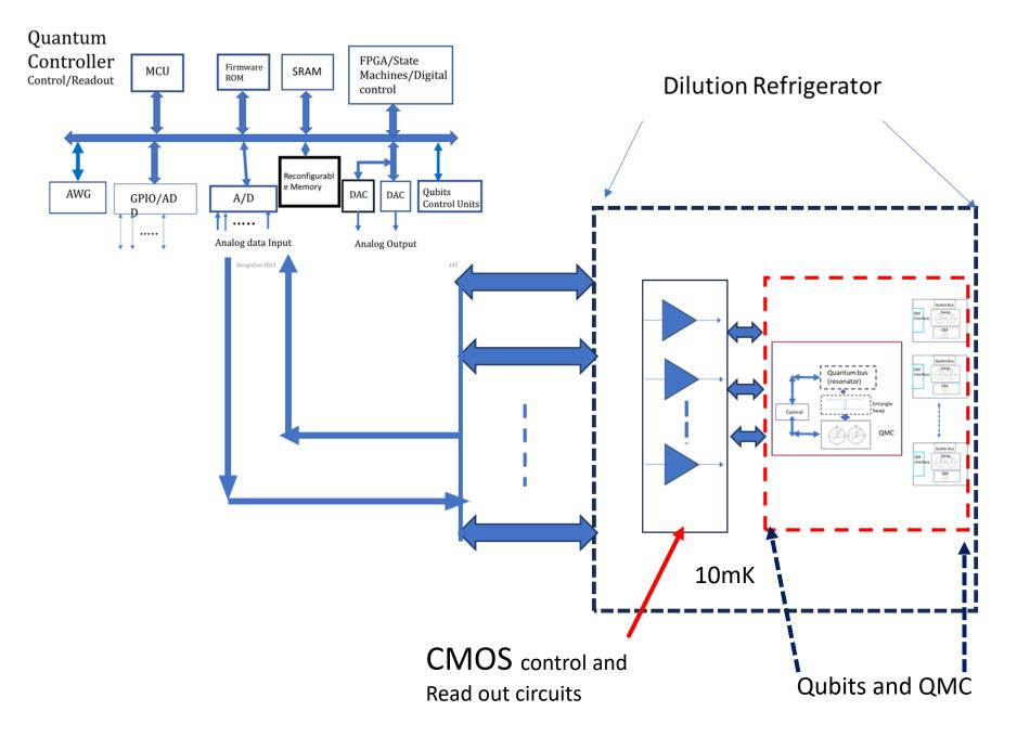
CMOS control and Readout circuits
