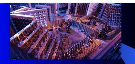
One possibility is to replace electrons with photons of laser light. One advantage is that light travels faster than electricity. The Chinese are leaders in this technology. But the collection of mirrors and beam splitters is quite complicated.
