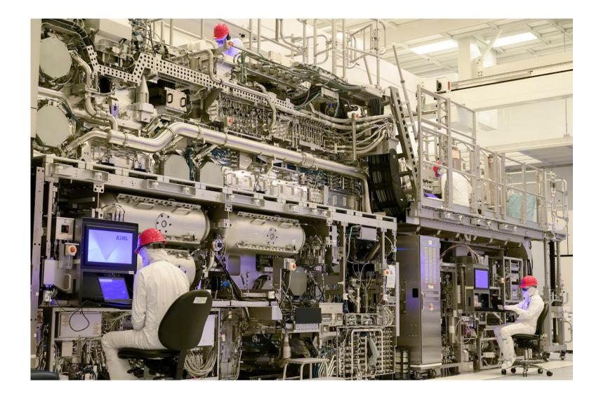
A High NA EUV manufacturing tool inside Intel's D1X research factory in Hillsboro.
