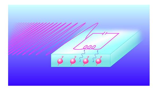
Superconducting circuit resonator and a silicon chip embedded with bismuth atoms. Chirped microwave pulses transfer quantum information back and forth between the resonator and the bismuth atoms, stored in the atoms spin states
