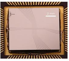
Surface-Electrode Trap Chip
