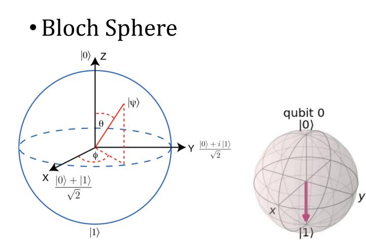
Superposition between |0>, |1>. The arrow is halfway between |0>, at the top, |1> at the bottom. Arrow can rotate to anywhere surface of the sphere.
