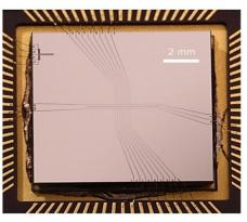
Surface-Electrode Trap Chip
