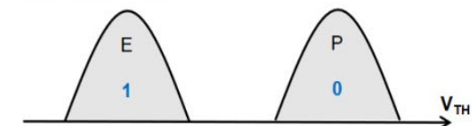
Single Level Cell (SLC): 2 States (1 Erase + 1 Pgm) = 1 bit of information per cell
