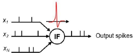
Spiking implementation allows for significant power reduction
