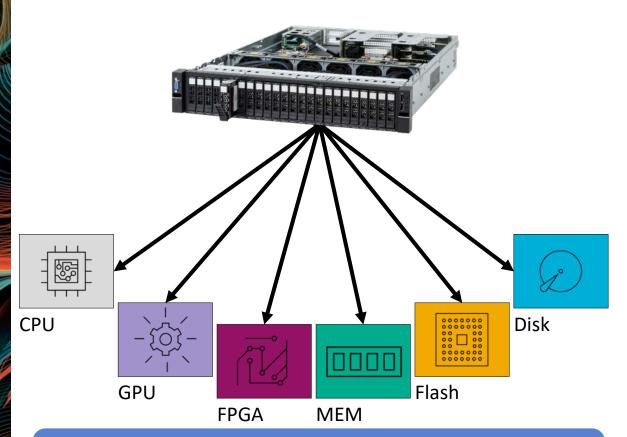
Disaggregate hardware components from the server so they can be efficiently pooled
