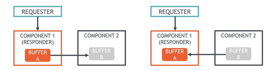
Gen-Z specifies 16 Buffer operations that simplify data movement, buffer allocation, security, etc.
