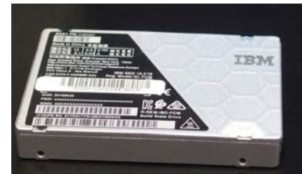
IBM's FlashCore™ Module (FCM) with STT-MRAM
