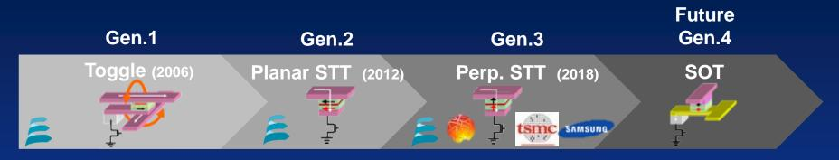
Not Scalable beyond 130nm (write power) Not Scalable beyond 65/40 nm (retention) Fully scalable Endurance-Retention-Speed tradeoff → Limited persistence and/or endurance and/or speed
