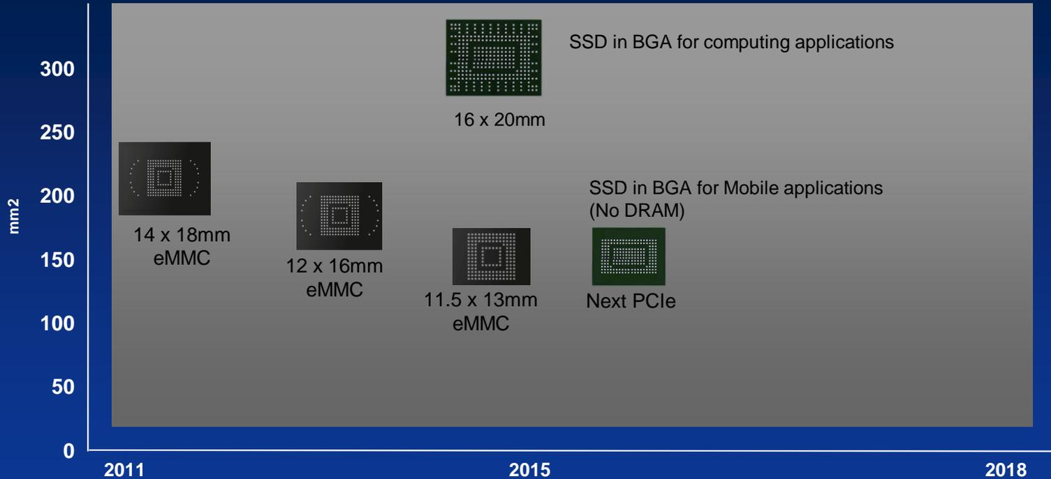
DRAM-less PCIe/NVMe SSDs can be packaged in 11.5 x 13mm
